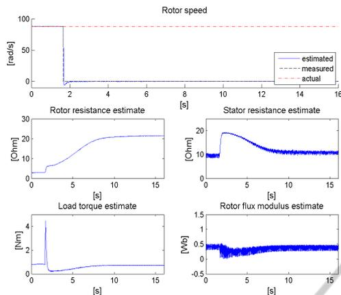
Figure 9: Third experimental test ( $\omega_m = 0$  rad/s,  $\omega = 88$  rad/s).
