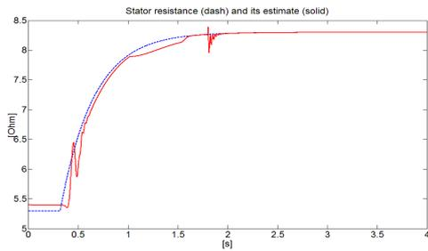
Figure 5: Stator resistance  $R_s$  (dash) and its estimate  $\hat{R}_s$  (solid).
