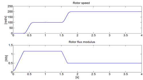
Figure 1: Rotor speed  $\omega$  and flux modulus  $\sqrt{\psi_{ra}^2 + \psi_{rb}^2}$ .
