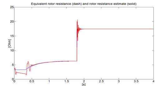
Figure 4: Equivalent rotor resistance  $R_{re}$  (dash) and its estimate  $\hat{R}_r$  (solid).
