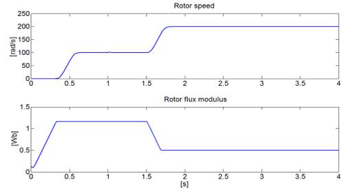
Figure 1: Rotor speed  $\omega$  and flux modulus  $\sqrt{\psi_{ra}^2 + \psi_{rb}^2}$ .
