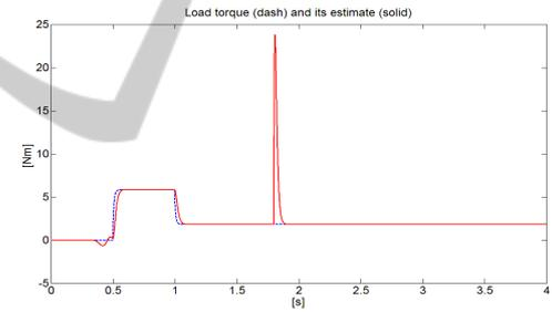
Figure 3: Load torque  $T_L$  (dash) and its estimate  $\hat{T}_L$  (solid).
