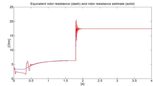
Figure 4: Equivalent rotor resistance  $R_{re}$  (dash) and its estimate  $\hat{R}_r$  (solid).
