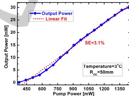
Figure 5: Average output power of the mode-locked laser at 3GHz repetition rate versus pump power at a temperature of 3°C.
