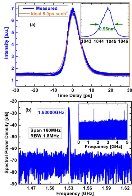
Figure 3: Measured and  $\text{sech}^2$  fitted autocorrelation trace (a) and RF spectrum (b) of the mode-locked pulses. The inset in (a) shows the optical spectrum and the inset in (b) shows the RF spectrum on a 5GHz span. The radius of curvature of the OC is 100mm.
