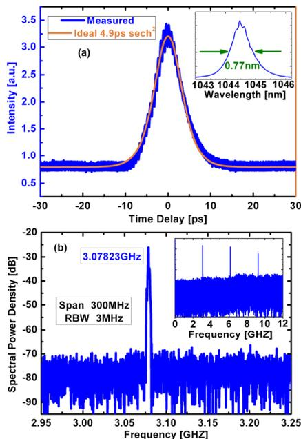
Figure 4: Measured and  $\text{sech}^2$  fitted autocorrelation trace (a) and RF spectrum (b) of the mode-locked pulses. The inset in (a) shows the optical spectrum and the inset in (b) shows the RF spectrum on a 12GHz span. The radius of curvature of the OC is 50mm.
