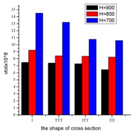
Figure 7: Volume comparisons of different cross section types.
