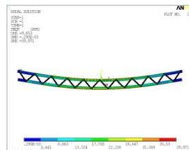
Figure 6: The deflection of the truss.
