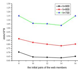
Figure 8: Comparisons of volumes with ITI cross section under different pairs of web members.
