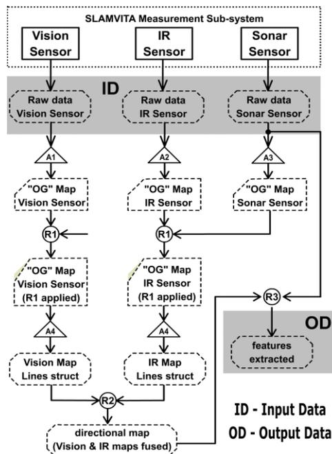
Figure 4: Flowchart of the proposed sensor data fusion algorithm.
