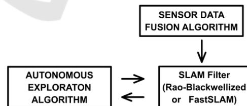
Figure 1: Algorithm modules to solve the indoor SLAM problem.
