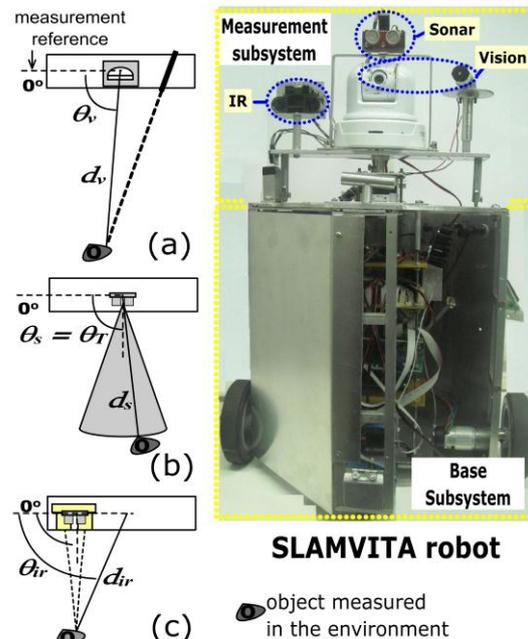
Figure 3: Measurement parameters ( $d$ ,  $\theta$ ) provided by the SLAMVITA sensors: (a) visual, (b) sonar and (c) infrared.
