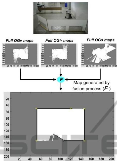
Figure 5: Comparison between OG maps computed from each sensor raw data and one generated by the proposed fusion algorithm.
