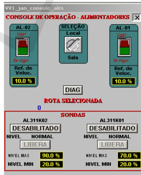
Figure 1: Manual adjustment of the feeders speed at VV01.
