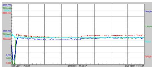
Figure 6: Comparison of the actual flow in ton/h (Blue) X Estimated Flow (Red) X estimated corrected flow (Green).
