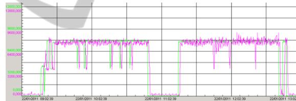
Figure 3: Comparison between estimated and actual flow.
