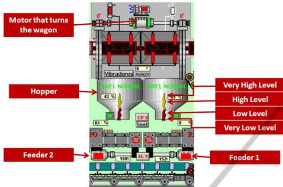
Figure 8: Monitors the level of ore in the hoppers.
