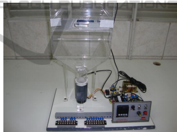
Figure 1: Educational kit for drying grains control.
