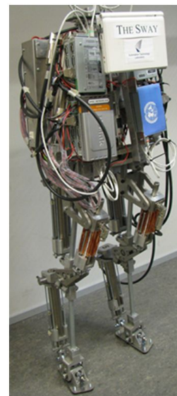
Figure 1: The SWAY, a bipedal autonomous walking robot.
