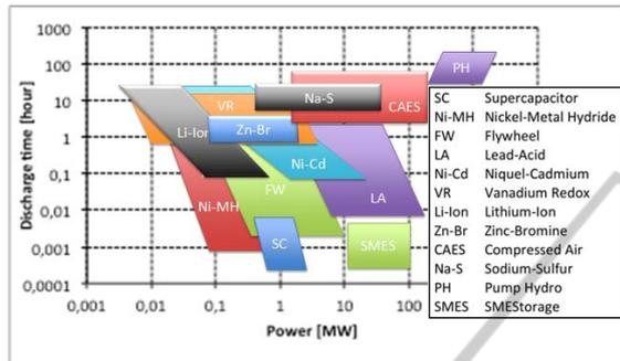
Figure 3: Comparison between ESS's power and discharge time.
