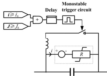
Figure 3: Electromagnetic model of FSC.
