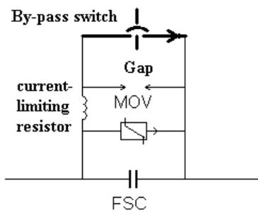
Figure 2: Schematic of FSC.
