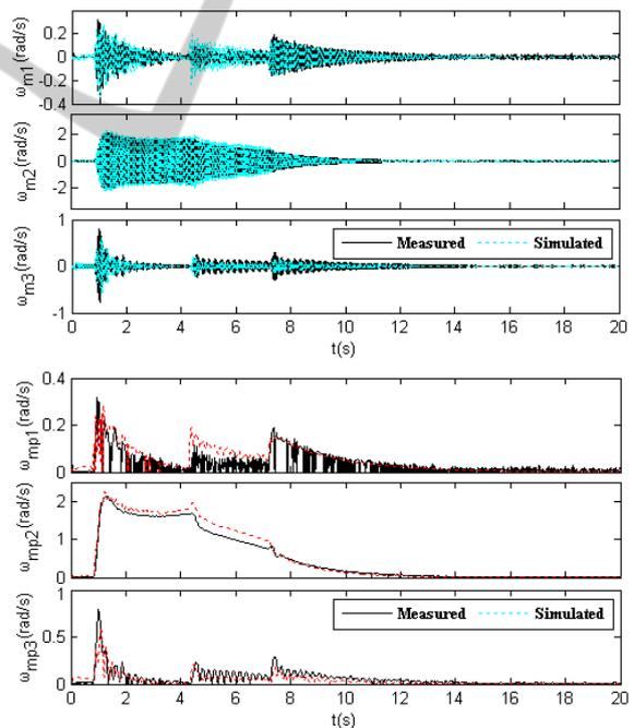
Figure 8: Measured vs. simulated SSR dynamics (unit #3).
