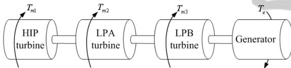
Figure 1: The lumped T-G shaft system.
