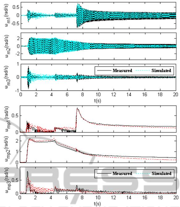
Figure 7: Measured vs. simulated SSR dynamics (unit #2).
