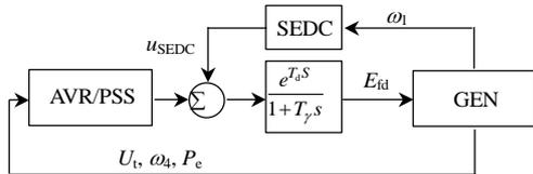
Figure 4: EMS model of the SEDC and excitation system.
