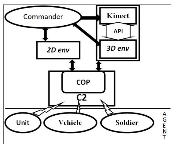
Figure 3: New architecture of C2 system with Kinect.
