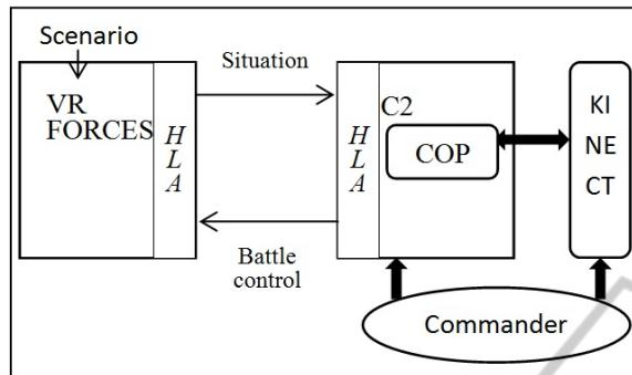
Figure 5: Operation control experiment architecture with Kinect.
