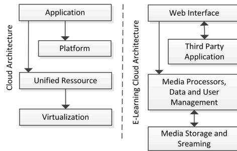
Figure 1: Cloud computing and e-learning cloud-based architecture.
