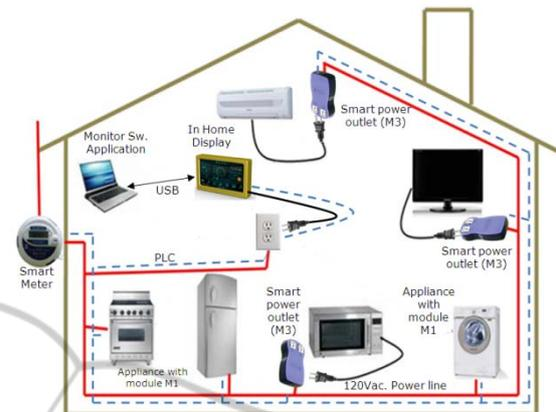
Figure 6: PLC communications network.
