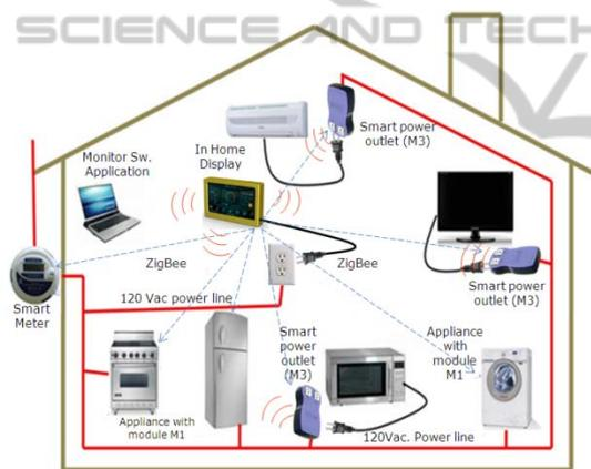
Figure 5: ZigBee communications network.
