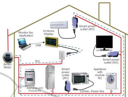
Figure 6: PLC communications network.
