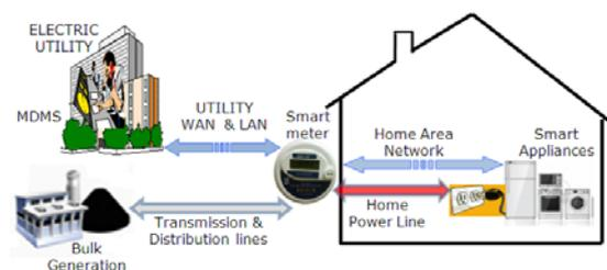
Figure 1: Simplified diagram of the operating environment of smart appliances in the context of smart grids.
