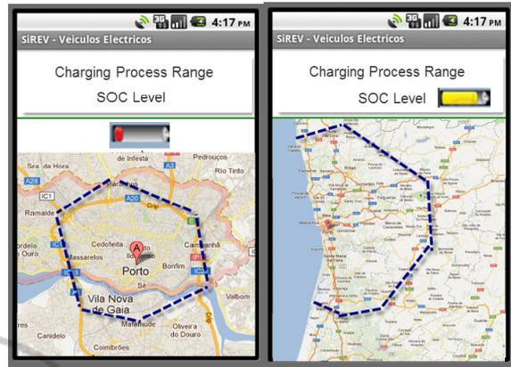
Figure 6: Representation of the charging range for different SOC levels, with a charging process performed in a public charging station in the centre of Porto city. On left, with a low SOC level, a small area is achieved. On right, with almost 90% of SOC level, a large area is achieved.
