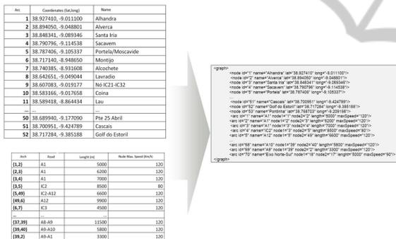
Figure 8: Semi-automatic creation of a XML file with road information to be used for graph creation.
