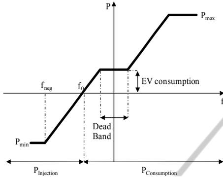
Figure 2: EV frequency-droop characteristic.
