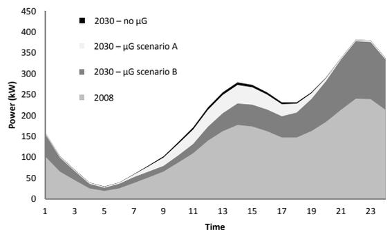
Figure 6: 2030 load diagram at the MV/LV substation of a LV network with 630 kVA transformer for the different scenarios of  $\mu$ G.
