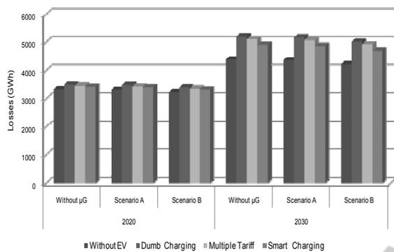
Figure 8: Total distribution network losses (MV and LV) for 2020 and 2030, High EV integration scenarios.
