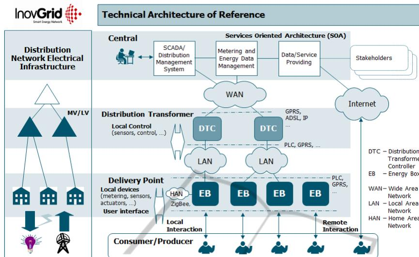
Figure 1: InovGrid advanced management and control system architecture.
