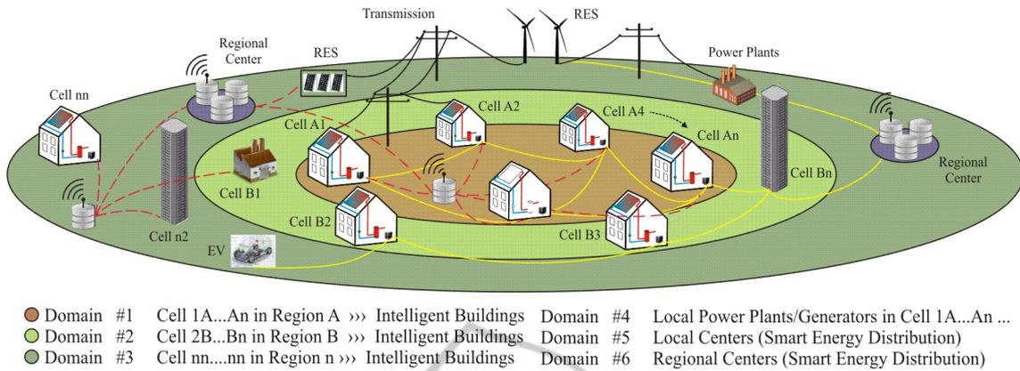
Figure 2: Overview of the smart energy distribution and power management with intelligent buildings.
