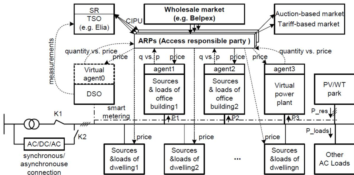
Figure 1: Architecture of a smart grid.
