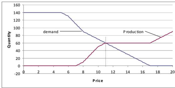
Figure 10: Power demand and production balance saturated at price=11 (reach maximal power production).
