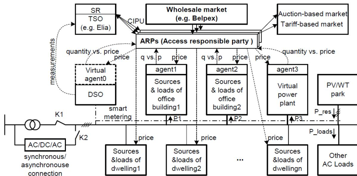
Figure 1: Architecture of a smart grid.
