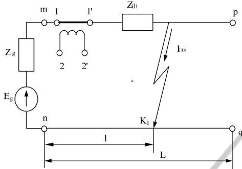
Figure 1: The scheme of detecting the cable fault point.  $L$  – cable length,  $l$  – distance from the beginning of the line to the point of short circuit,  $E_G$  – system EMF,  $Z_G$  – internal resistance of the system,  $Z(l)$  – resistance of the line section from its beginning to the short circuit location.
