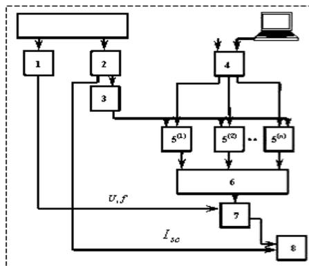
Figure 2: Structural scheme of on-line determination of the short circuit point on the transmission line.
