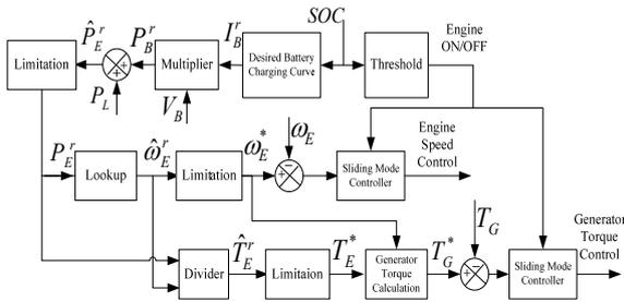
Figure 2: Proposed powertrain control system.
