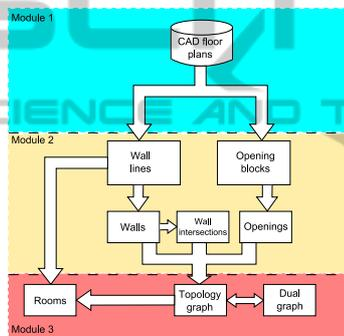
Figure 1: Framework based in a three-level architecture to represent building information models.
