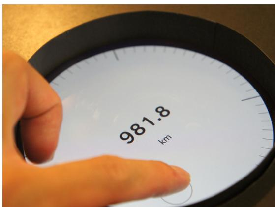
Figure 2: The dial for setting distance.
