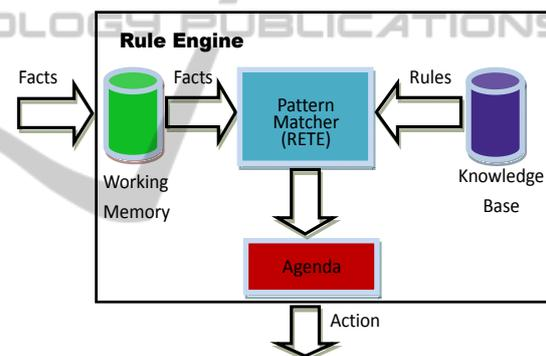
Figure 1: Basic architecture of rule engine.
