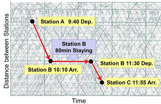
Figure 2: The transfer process with diagram.
