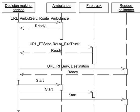
Figure 6: Emergency responders accept emergency response plan.
