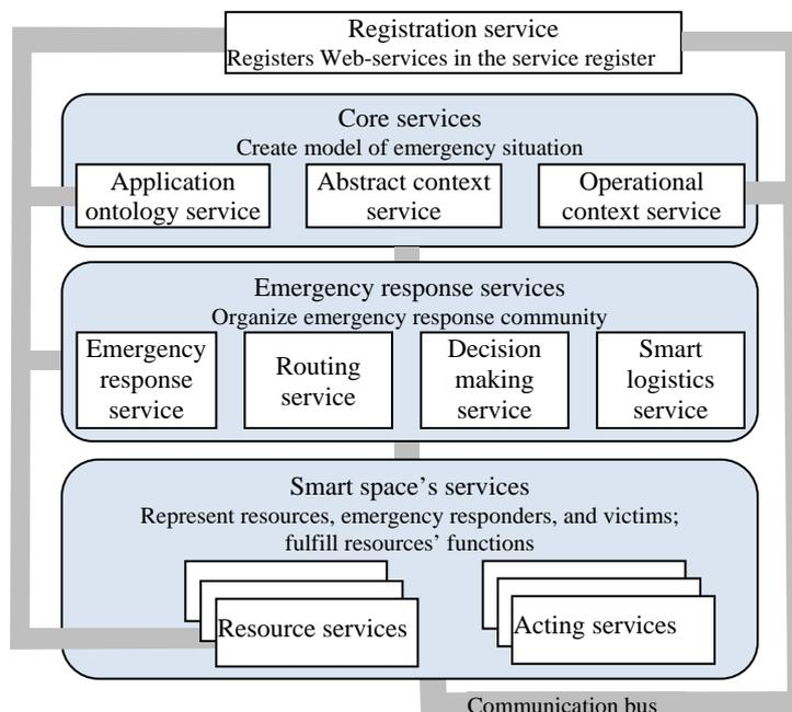
Figure 5: Service-oriented architecture.
