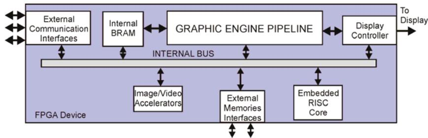
Figure 1: Graphic acceleration system on FPGA.
