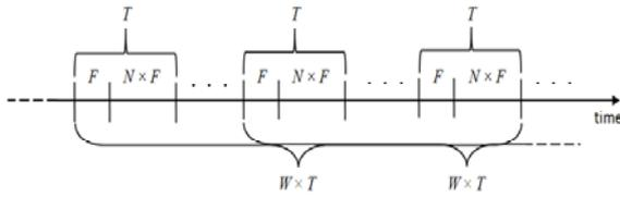
Figure 1: Diagram representing the raw accelerometer signal acquisition.
