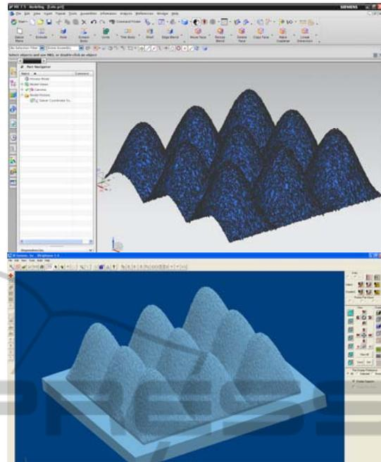
Figure 2: Handling the surface with CAD software for obtaining a solid model.
