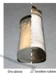
Figure 2: Swelling behaviour of the nanostructured hybrid scaffold material.
