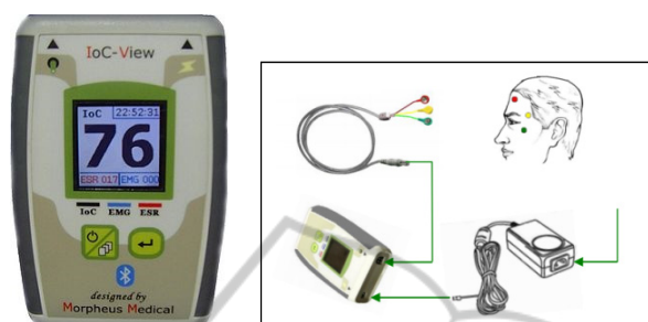
Fig. 1. IoC-View monitor (Aircraft Medical (Barcelona), Barcelona, Spain), shown on the left. The techniques for connection of electrodes to the monitor and placement of the electrodes on the forehead of a human patient are shown on the right [13].
