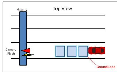
Figure 2: Top view of the experimental testbed.
