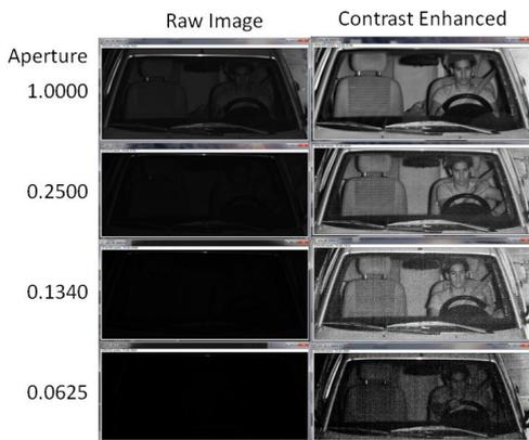
Figure 4: Vehicle images at various aperture settings. Raw images and contrast enhanced.
