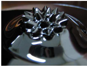
Figure 2: Spiking phenomenon of magnetic fluid (photograph).
