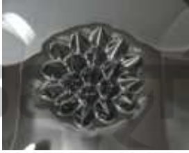
Figure 5: Photograph of a real magnetic fluid surface.
