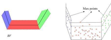
Figure 2: Reconstruction process: (a) buffer regions surrounding footprint (b) max height point extraction.
