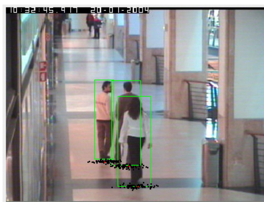
Figure 6: Frame with target bounding boxes and projection of particles on camera plane (points near the base of the targets). The upper two pedestrians are walking together.
