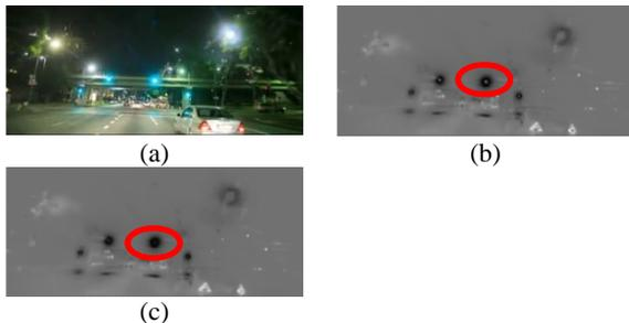
Figure 4: Handling the “blooming effect” at night. (a) RGB image, (b) RGYB channel, (c) RGYB channel after filling process.
