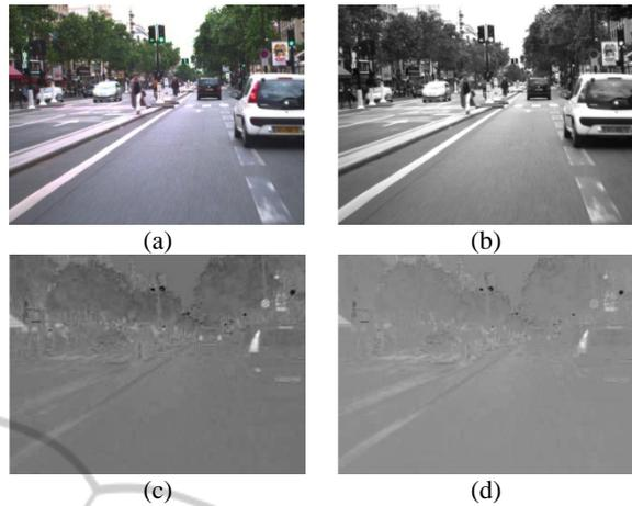
Figure 2: Red-green discrimination enhancement. (a) RGB image, (b) L channel, (c)  $a^*$  channel, (d) L,  $a^*$  multiplication result (RG channel).
