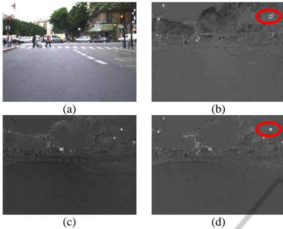
Figure 3: Handling the “blooming effect” in the morning. (a) RGB image, (b) RG channel, (c) YB channel, (d) RGYB channel.
