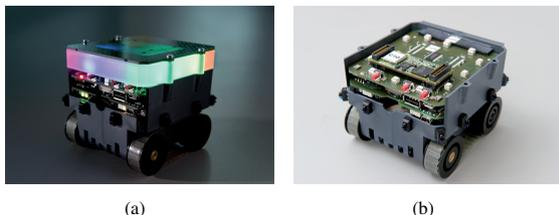
Figure 1: Miniature robot BeBot, (a) with and (b) without light guide, enabling the robot to express its internal state.
