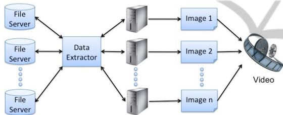
Figure 3: Overview of the Spiegel framework. Data is extracted from one or more file servers and distributed to a cluster of computers. Each processing unit in the cluster generates one (or more) frames of the complete visualization sequence in parallel. These frames are then combined to create a video. Image courtesy of (Espinal et al., 2010).
