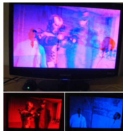
Figure 4: Stereo video player for two users. Top, photograph of the monitor, showing both videos. Bottom, viewing the monitor through a red filter and blue filter.
