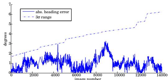
Figure 7: Absolute heading error and  $3\sigma$  range without adjustment.
