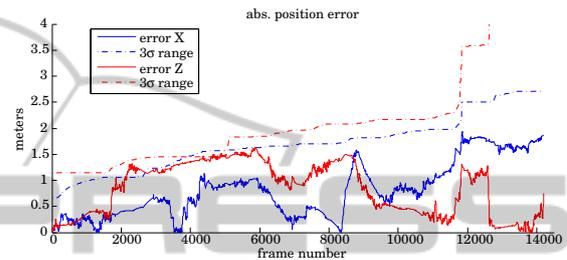
Figure 6: Absolute position error and  $3\sigma$  range without adjustment.
