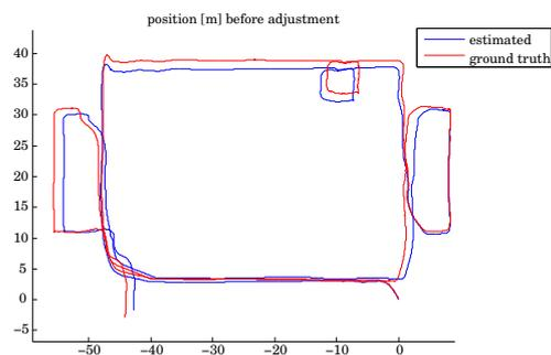
Figure 8: Estimated trajectory in [m] without adjustment.
