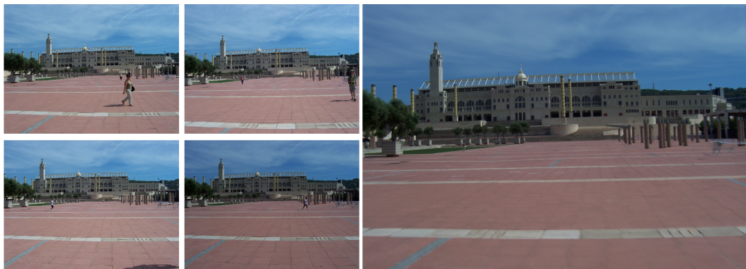
Figure 5: Result from 8 pictures using a low budget camera. This set contains a lot of translations and rotations. The result is sharp, which demonstrates the correct registration of the images. Notice that the clouds are washed out, but are still plausible.
