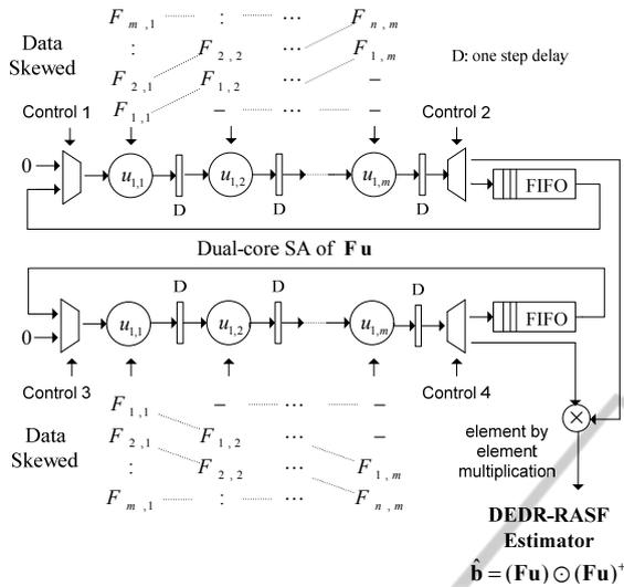
Figure 1: Dual-core SA for the DEDR-RASF estimator.
