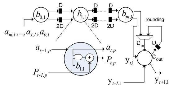
Figure 3: Bit-level SA of the MAC structure.
