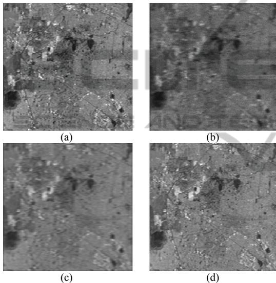
Figure 4: Results of the HW/SW co-design implementation for SAR images with 15dB of SNR: (a) Original test scene; (b) degraded MSF-formed SAR image; (c) RSF reconstructed image (IOSNR = 7.49 dB); (d) RASF reconstructed image (IOSNR = 9.14 dB).
