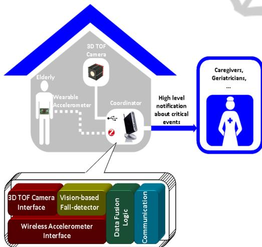
Figure 1: Overview of the multi-sensor system in which the information coming from the wearable accelerometer module and the TOF camera is combined by the coordinator node in order to reliably detect falls.
