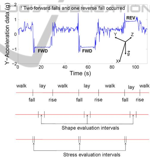
Figure 9: Acceleration data stream session measured along Y-axis with wireless device worn on the belt. The Y-axis is orthogonal to the belt.
