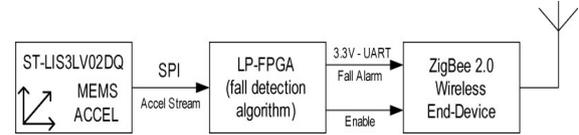
Figure 5: Block diagram of the developed wearable wireless accelerometer hardware.
