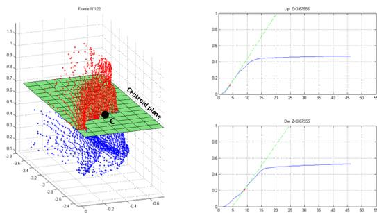
Figure 3: 3D point cloud of a posture (Sitting) and the related upper and lower volumetric point distributions.
