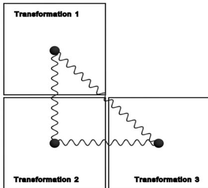
Figure 1: The model of IFS representing rigid bodies connected with springs.
