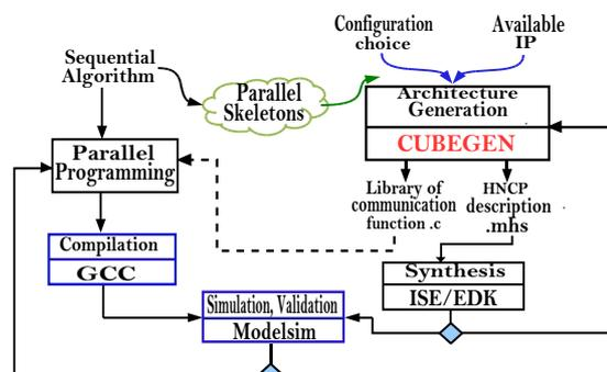
Figure 5: The proposed design flow.
