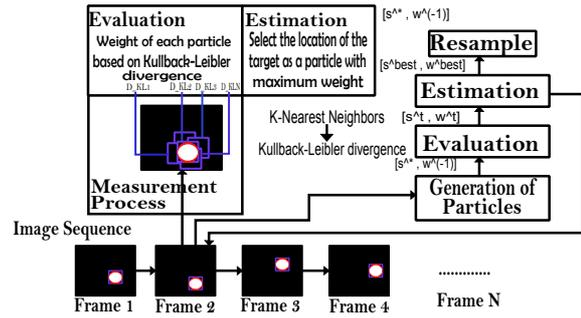
Figure 2: Particle filter scheme.
