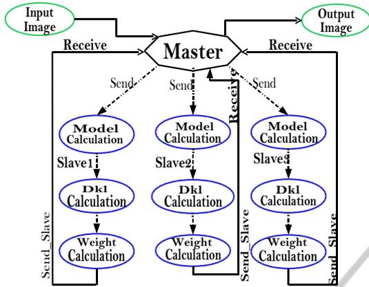
Figure 7: Parallel face tracking using FARM (case of HNCP with 4 processors).
