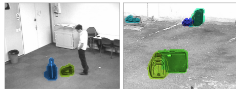
Figure 1: A mask is used for each label to store the stationary objects. Thus, we know which are the visible and occluded parts of each object. The visible parts of stationary objects are coloured.
