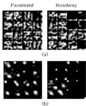
Figure 8: Texture feature of pavement and roadway, (a) 8x8 window blocks based rotation invariant LBP, (b) 8x8 window blocks based GLCM.
