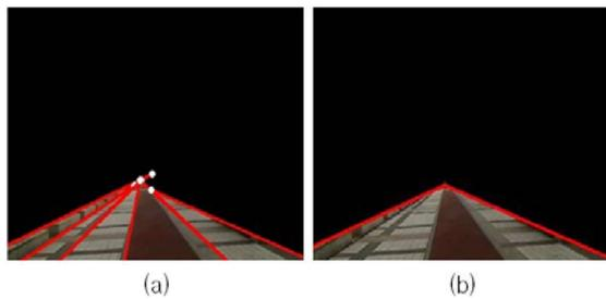
Figure 5: Separating the ROI and extracting a single triangular model, (a) primary interested regions, (b) the merged triangular model region.
