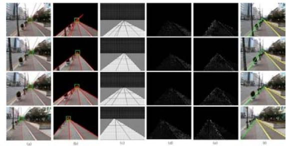
Figure 11: Process of texture feature extraction in real time image: (a) valid hough line detection, (b) region of triangular model, (c) separated according to 8x8 window block (d) rotation invariant LBP in triangular model, (e) GLCM in triangular model, (f) pavement and roadway detection result.
