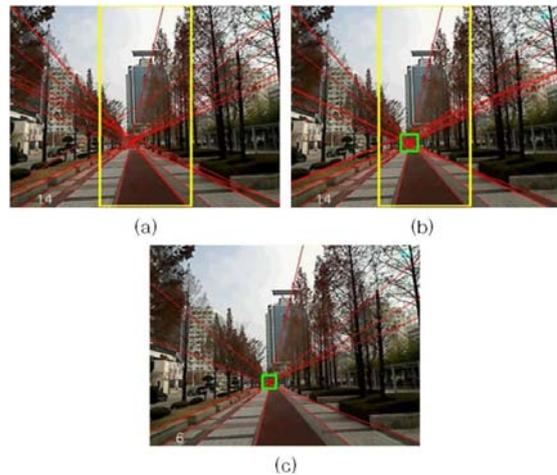
Figure 4: Process of detection for valid vanishing line, (a) the candidate region for the location of the vanishing point, (b) improved Hough line after eliminating invalid lines, (c) optimal valid vanishing lines.
