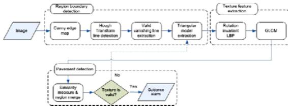
Figure 2: Pavement detection framework.
