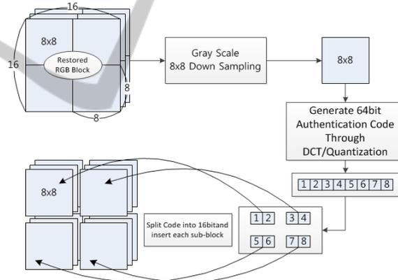
Figure 2: Authentication code generation and splitting.
