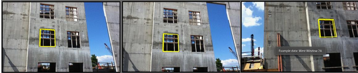
Figure 1: Screenshots of the android HD<sup>4</sup>AR client overlaying bim information related to a window.
