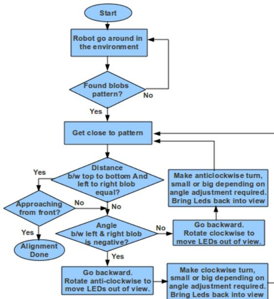
Figure 4: Flow diagram of control algorithm.
