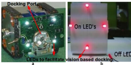
Figure 2: (a) Docking port and LEDs to facilitate vision based docking. (b) Dummy docking port.
