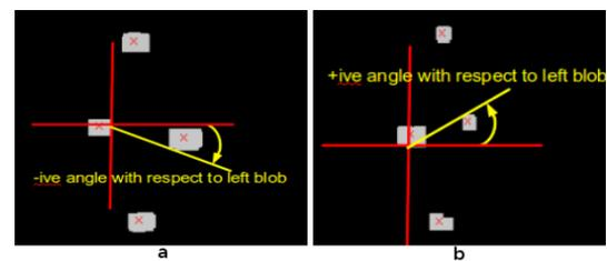
Figure 5: (a) Robot approaching from left side. (b) Robot approaching from right side.
