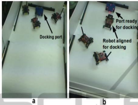
Figure 9: (a) A collective search for docking port (b) One robot finds the docking port and the rest quit mission.
