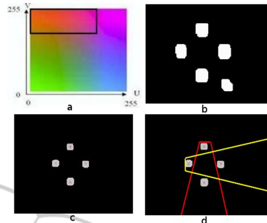
Figure 3: (a) UV plane. (b) Output of blob detection algorithm. (c) Blob statistical information. (d) Search field for neighbouring blobs.
