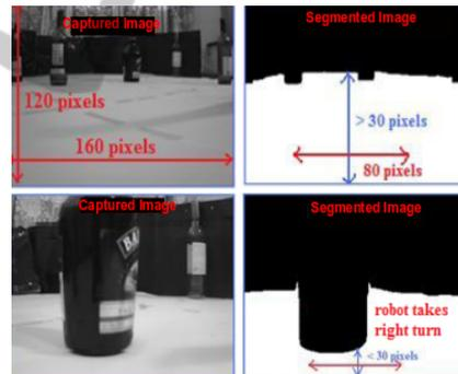
Figure 5: Segmentation based obstacle avoidance.
