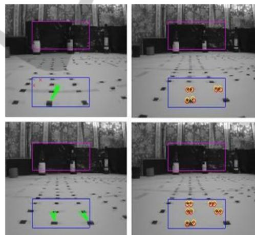
Figure 9: Lucas-Kanade and Normalised cross correlation feature tracking and matching results.
