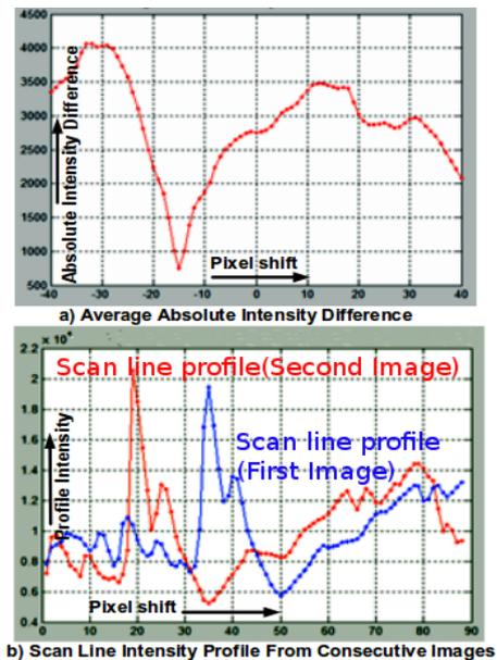
Figure 4: a) Average intensity difference when one profile shifted over the second. b) Two scanline profiles.
