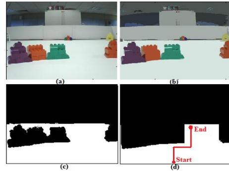
Figure 2: The step by step processing of segmentation based obstacle avoidance algorithm.
