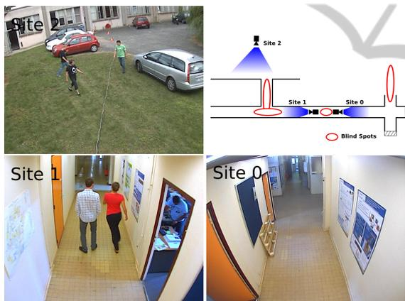
Figure 2: Camera network with non-overlapping fields of views.
