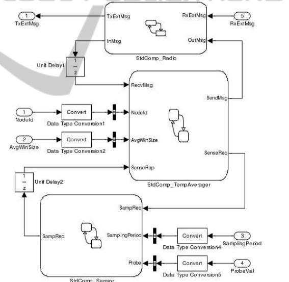
Figure 8: Node applications composed of linked blocks.
